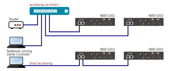
The network interfaces of the NBB Series products are by default configured to work in auto-IP mode. If your network does not has a DHCP server or router involved, you may have to configure the IP of your computer in the range of 169.254.xxx.xxx to have your computer talk to NBB Series products.
