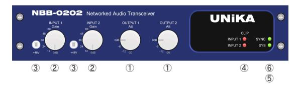
To accommodate all the variety of field installation, the front panel of NBB Series Products is equipped with rich control facilities as follows,
