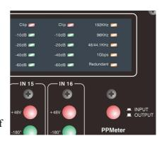
Besides measuring input audio, you are able to switch all the 16 meters to monitor level on output by simply pressing an INPUT/OUTPUT button on the far right of the front panel.
