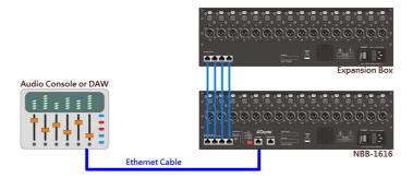
Daisy-chain With the two network ports configured to work in switch mode, you can cascade several NBB-1616s in a same link. This greatly simplifies the network wiring and devices deployment if you need to route audio to several spots sequentially.
