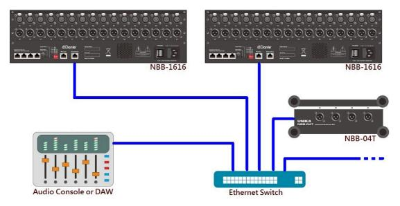
**System Scaling Up** Computer network can be further expanded with more than one Ethernet switch, so does NBB-1616 audio network. You can use more than one switch between NBB-1616s to greatly expand your audio distribution.
