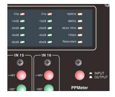
Besides measuring of input audio, you are able to switch all the 16 meters to monitor level on output by simply pressing an INPUT/OUTPUT button on the far right of the front panel.
