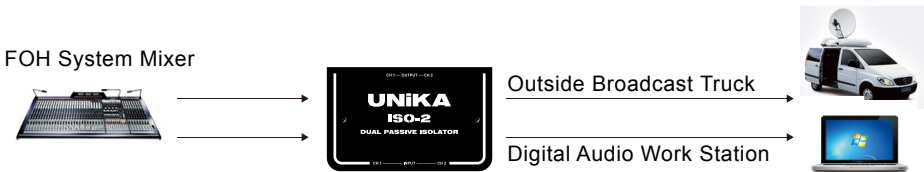
Fig-6: Mixing console to devices with different power source
